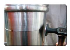
Peen the tacked joint to ensure correct fit.
