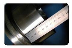
If it is necessary to shorten the tail, do not cut the tail more than 1" (25mm) unless absolutely necessary. Welding any closer than 1" (25mm) to the head, could result in welding shrinkage effecting the tolerance of fit between the flexible connector cuff into the BFM® fitting. Consult Siftex prior to cutting.
