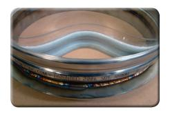
Be careful to ensure that the circumference of the formed end after fitting and welding, remains the same size as supplied, to ensure fitting tolerance of the connector.
